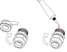
CAUTION: Teflon tape and some pipe sealants are destructive to hydraulic components. Always use extreme caution and follow manufacturer's recommendations for proper application of any sealant in order to prevent contamination.
