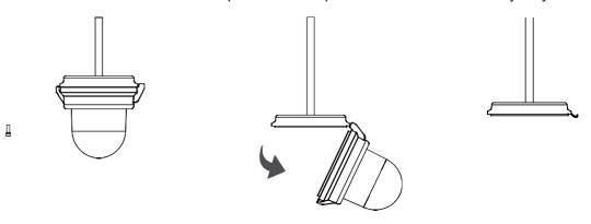
STEP 2: Thread the male-to-male connector onto the retrofit adapter and fixture; Tighten the M4 set-screw.
