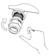
**STEP 4:** Wrench tighten the fitting to the correct Turns Past Finger Tight position. A properly assembled fittings total thread engagement should be 3.5 to 6 turns.
